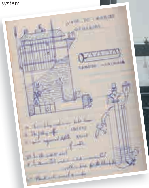
Below: Notes and sketches from Tommy Purcell's workbook from his courses in Bolton Street c. 1940s. Diagram of low pressure heating system.
